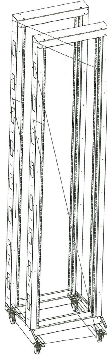
**Step 3:** Attach the frames to the support beams where the castors are attached. The server rack is ready for use now
