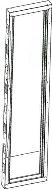
**Step 1:** Attach the vertical rails together with the L-shaped support beams to make 1 frame
