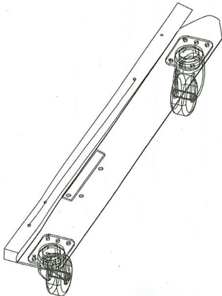
**Step 2:** Attach the castors under the support beams
